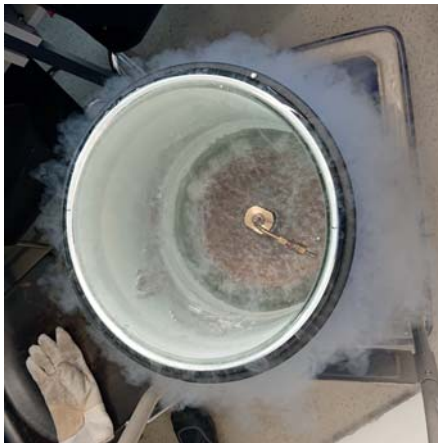
Figure 2: Deep-freeze test chamber with vacuum connection
