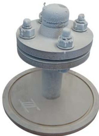
Figure 3: Deep-freeze test flange
